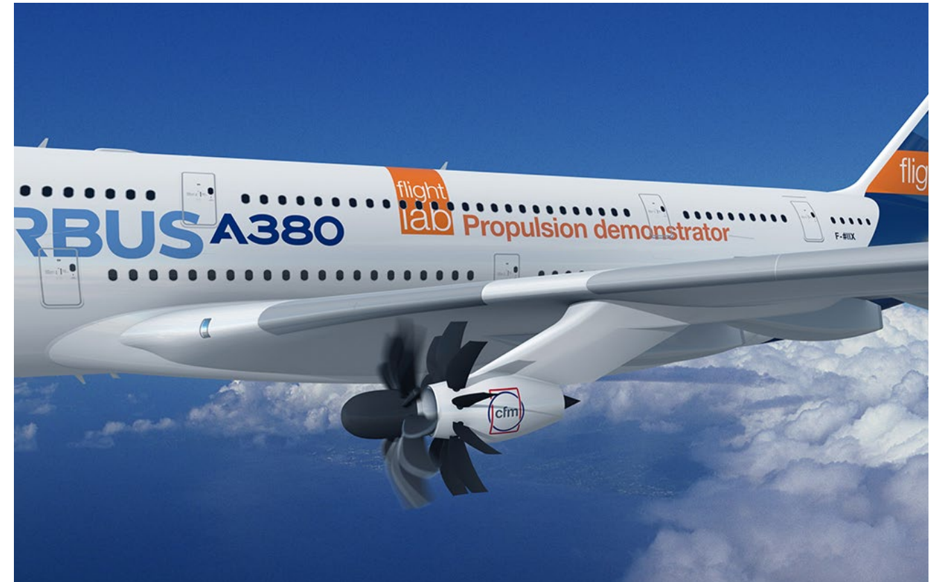
CFM International and Airbus plan to flight test Open Fan engine architecture this decade. Image credit: Airbus.
