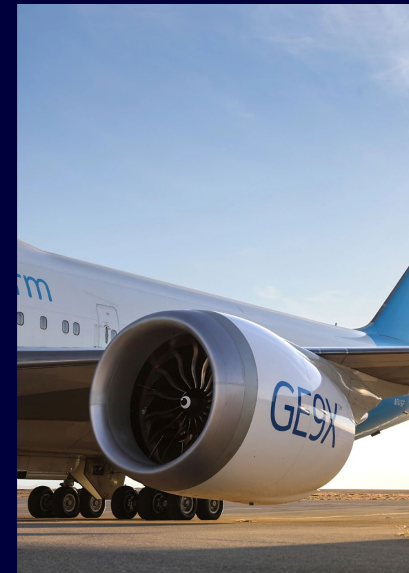
GE9X engine installed on GE Aerospace's flying test bed.
