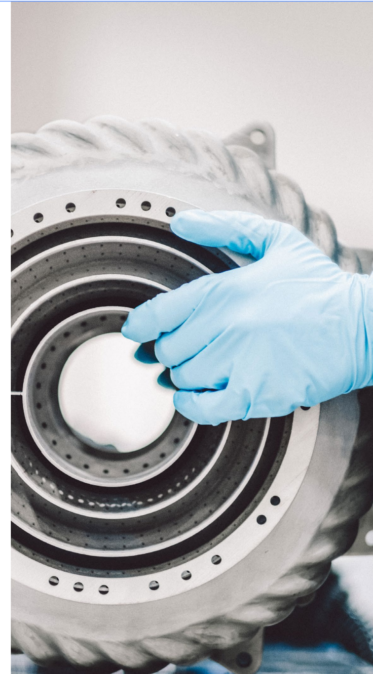
Additively manufactured mid-frame structure for an A-CT7 concept engine.
