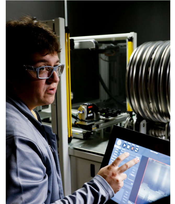
The Deep Cavity Inspection System is a fully automated, enhanced surface inspection solution for finished and fielded engine spool assemblies.
