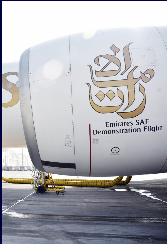
GE Aerospace's GE90 engine powered a demonstration flight in 2023 with 100% SAF in one of the two engines. Image credit: Emirates.
